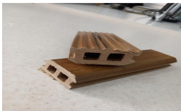
Figure 1. Experimental sample of wood polymer composite material based on PVC and wood waste
