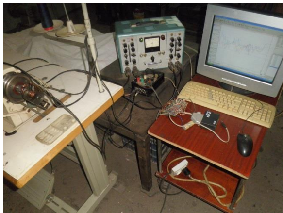
Fig.1. A general view of the experimental installation of a sewing machine with an advanced presser foot design with an additional spring.
