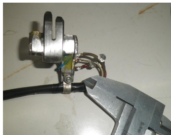
Fig.4. General view of the foot with the foot movement control sensor.
