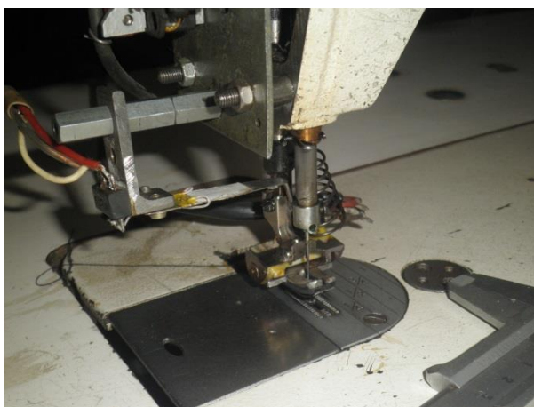
Fig.4. General view of the foot with the foot movement control sensor.
