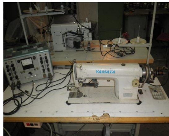
Fig.1. A general view of the experimental installation of a sewing machine with an advanced presser foot design with an additional spring.
