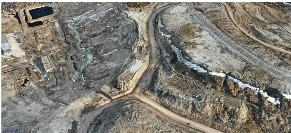
Figure 4. Constructed dense point cloud of photographs obtained during shooting from a quadrocopter in the Agisoft PhotoScan program
