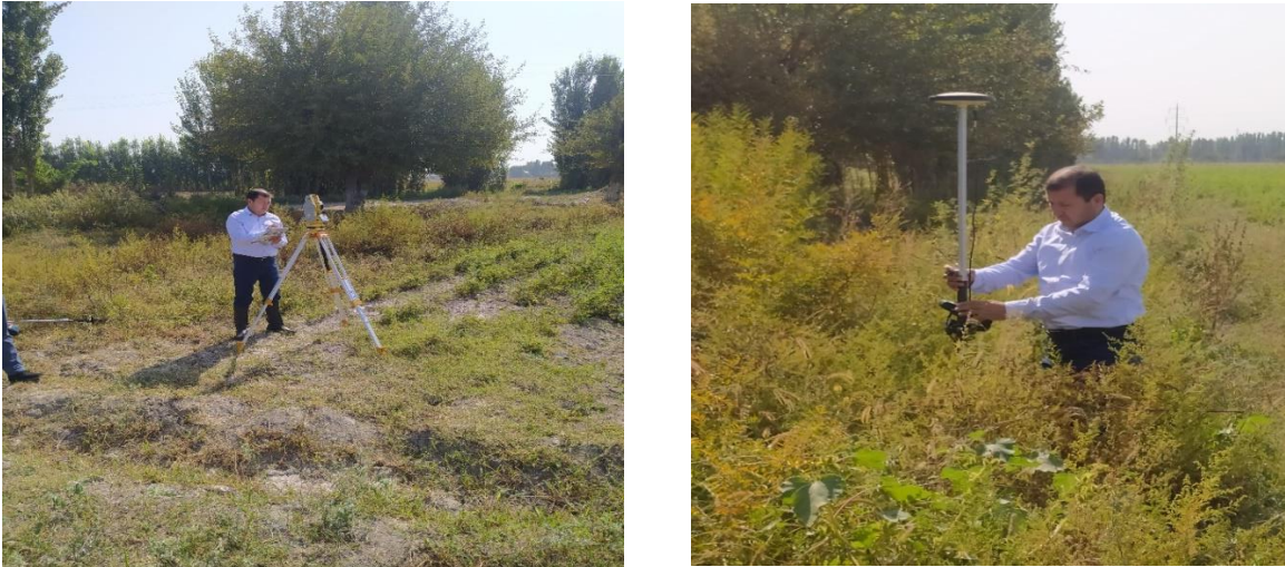
Figure 4. Land area measurement process by using an electronic tacheometer and GPG
